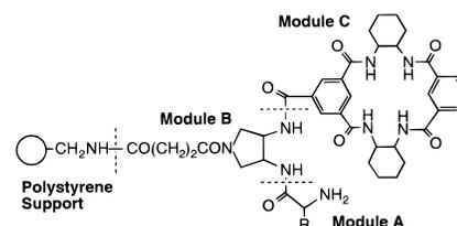
The library was prepared by encoded split synthesis on 100  $\mu$ m polystyrene synthesis beads; thus, different library members were segregated on different beads (i.e., one bead, one chiral selector).<sup>10</sup> Details are given in the Supporting Information.
