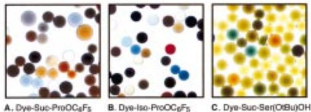
**Figure 1.** Chiral selector library beads screened for enantioselective binding by treatment with differentially labeled enantiomeric amino acid derivatives.
